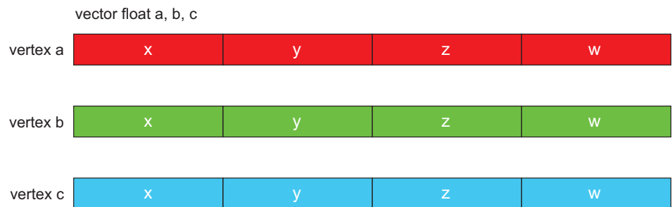
Figure 24. Array-of-structures data organization for one triangle
